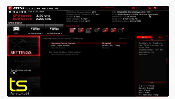
• Usually, TPM is in the same section. You should also disable it. For some machines, it disables simultaneously with Secure Boot.
